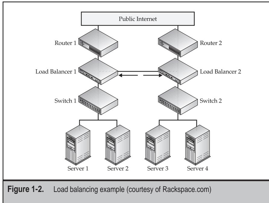
Figure 1-2. Load balancing example (courtesy of Rackspace.com)
